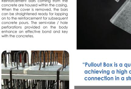
"Pullout Box is a quick and safe method of achieving a high quality reinforcement connection in a structural concrete joint"
